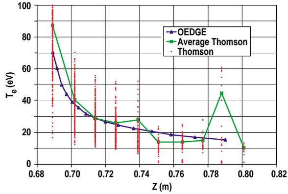
Fig. 6. Comparison of  $T_e$  profile along the vertical line of the upstream Thomson system, see Fig. 1. The points are the Thomson values for 5 of the low density SAPP shots. Also shown is the average value of the Thomson data as well as the OEDGE result. The contributions of the individual onion-rings to the OEDGE solution are evident. The error estimates for the  $T_e$  values varies from 10% to 80%, with an average of 35%.
