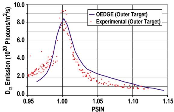
Fig. 8. Comparison of the filterscope  $D_\alpha$  profile across the outer target (obtained with sweeping of the X-point, and by combining data from several filterscope channels) with the OEDGE (EIRENE) result.
