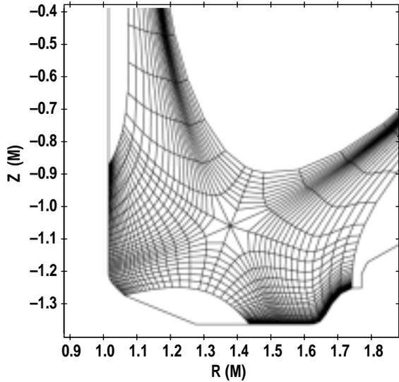
Fig. 3. Computational grid showing poloidal flux surfaces, i.e. “onion-rings”. The particular rings used in Figs. 4, 5, – rings 10, 12, 14, and 16 – have normalized magnetic flux values  $\psi_n = 1.00148$ ,  $1.00737$ ,  $1.01431$ , and  $1.02327$ , respectively. Ring 10 is closest to the separatrix and the rings radially further out have larger numbers.
